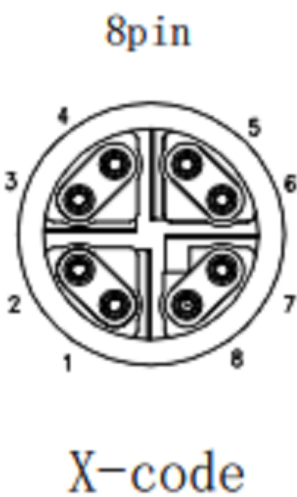
Pin assignment front view/针位分布前视图
